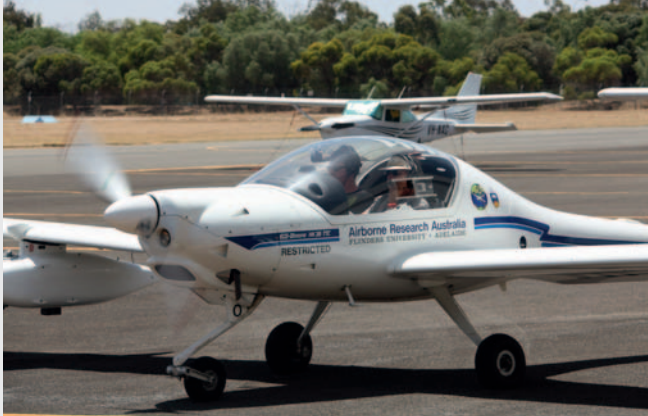
Dr. Andreas Backhaus starting with an aircraft to record hyperspectral images of vineyards near Adelaide. The camera is in a housing mounted on the underside of the wing (to the left). Photo: Udo Seiffert
