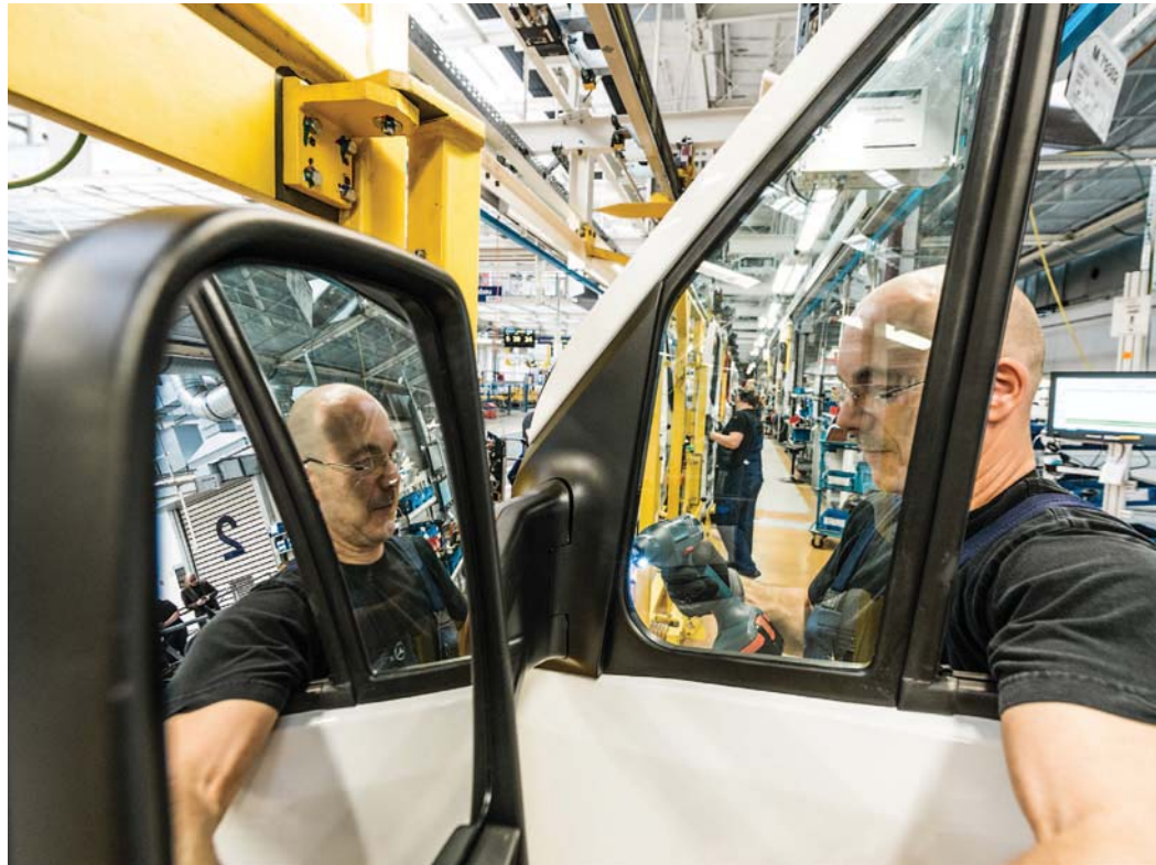
Installing side view mirrors on light commercial vehicles is not always easy because of the wide variety of models. Outwardly, the mirrors are virtually indistinguishable. Photos: Fraunhofer IFF, Andres Süß
