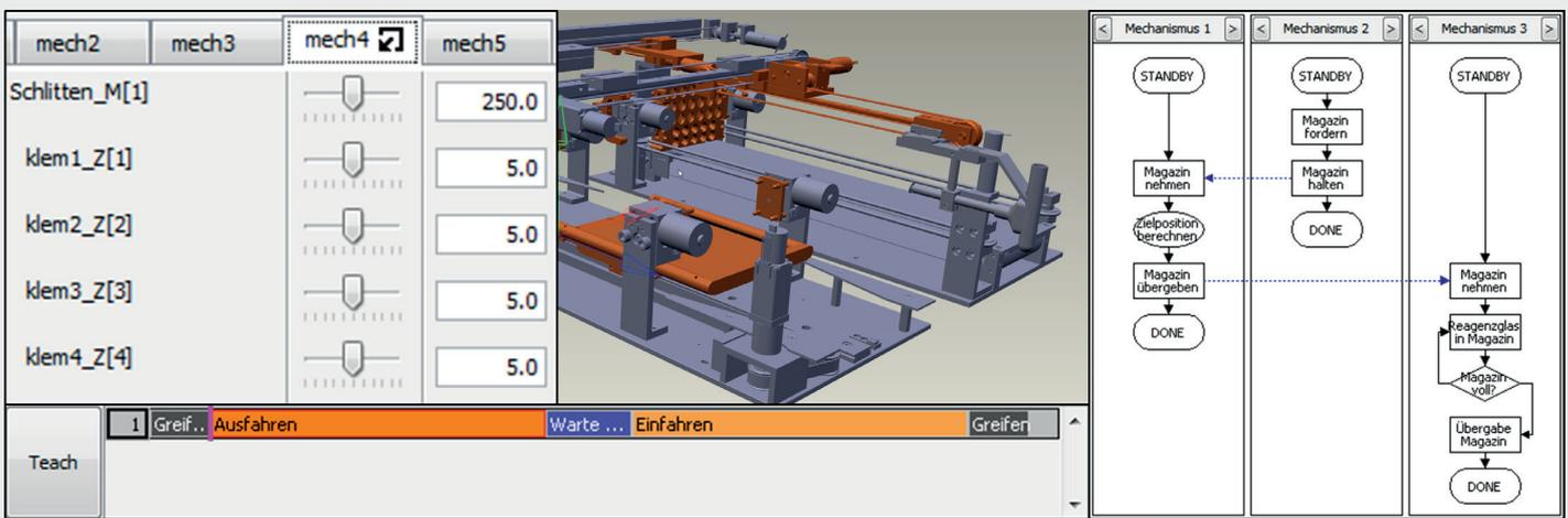
Along with cutting the time required for programming and commissioning significantly, VINCENT most notably facilitates integrated development of custom machines. Immediate testing of control code on a virtual machine validates programming early on.
