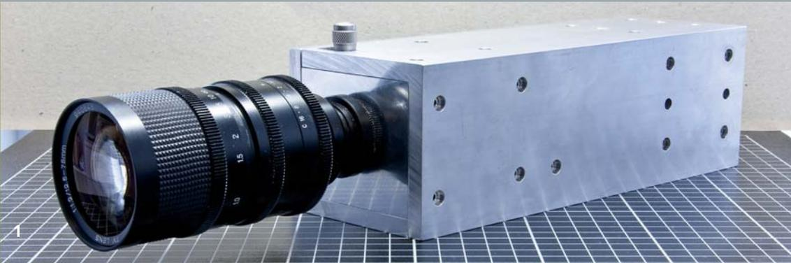
1 HawkSpex®, a flexibly configurable hyperspectral camera. Photo: Udo Seiffert
