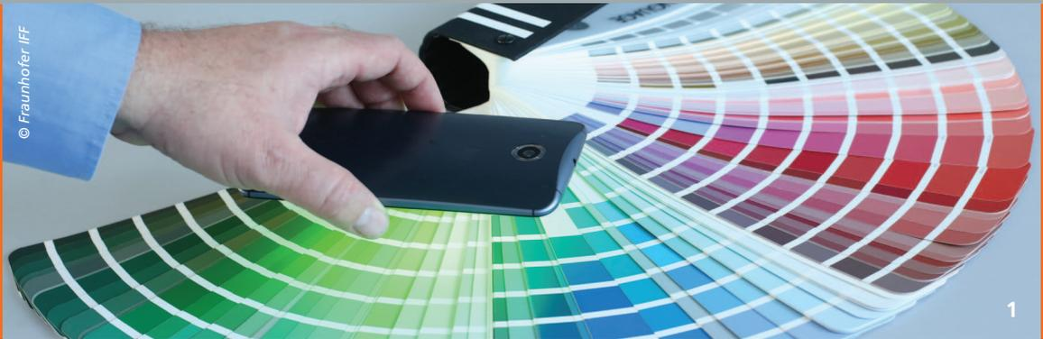
1 A smartphone spectrometer– made possible without additional hardware by HawkSpex® Mobile.
