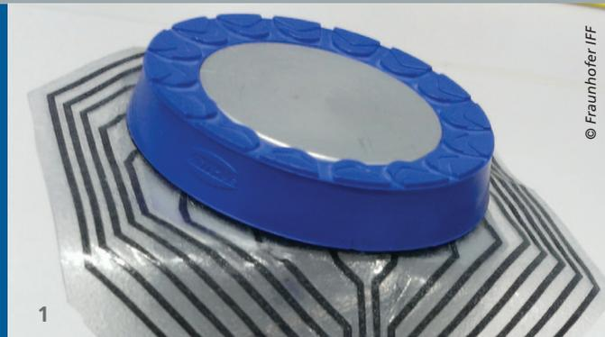
1 Object pose as determined by a magnet gripper with a tactile sensor.
