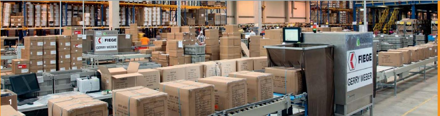
1 RFID Tunnel Gates in use at FIEGE Megacenter in Ibbenbüren.
