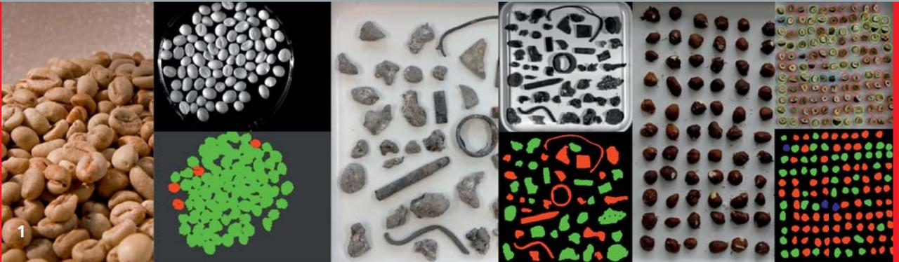
1 Classification of different materials from recycling, coffee grading and nut inspection – the outcome of the Fraunhofer IFF's soft sensor solutions.
