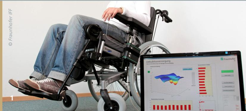
1 Use case: *Sitting pressure sensing in a wheelchair.* Photo: Dirk Mahler, Fraunhofer IFF
