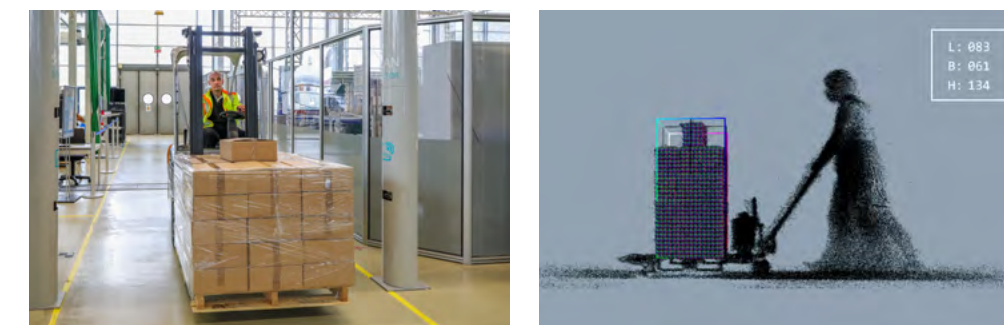
Figure 10: Pallet scanning with 3D sensors, Workshop 2
