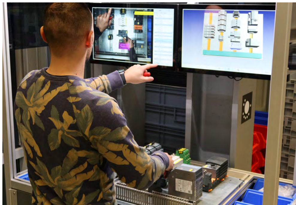
Figure 9: Assistance and inspection system for the installation of control cabinets, Workshop 2
