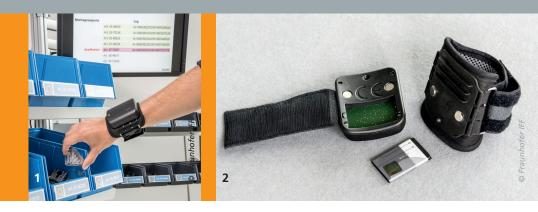
1 The RFID Wristband identifies objects or picking areas during handling operations.
