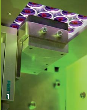
1 Level metering with clamp-on technology.
