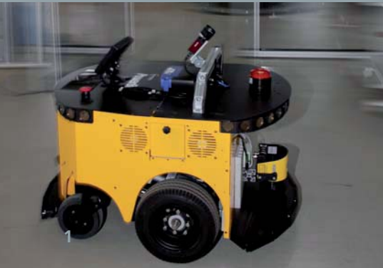
1 Mobile robot with visual navigation.
